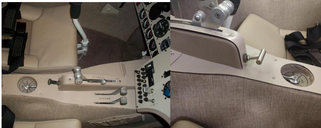
Normal choke with throttle friction shown at left. Modified choke T handle was added for easier choke operations shown on the right.
