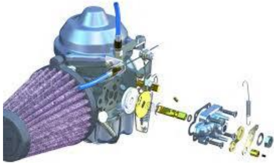
Modified straight choke cable adapter for the Bing 64 on a Kitfox.
