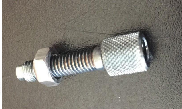
Modified straight choke cable adapter for the Bing 64 on a Kitfox.
