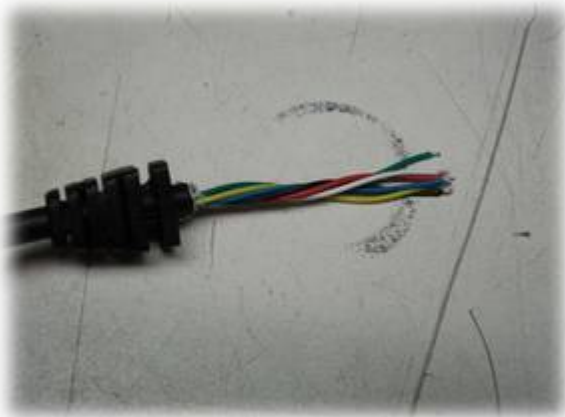
New cable with strain relief (Photo 5)
