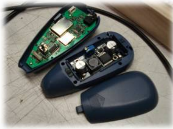
DC-DC converter in battery compartment (Photo 2)
