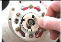
Remove the card spacer noting its orientation.
