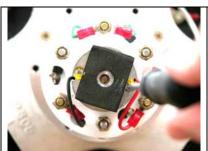
Unscrew the two screws holding the top of the PC motor on. Note: use Loctite 243 in thread when reassembling.
