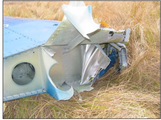
R/H wing: main spar failure
