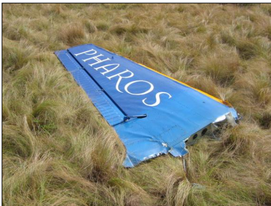
R/H wing: lower surface
