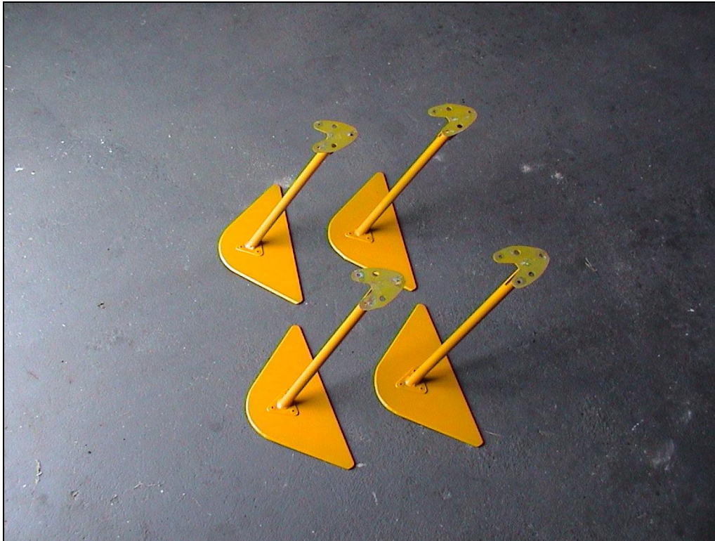
Aileron spades / mass balances later discovered in the hangar.
