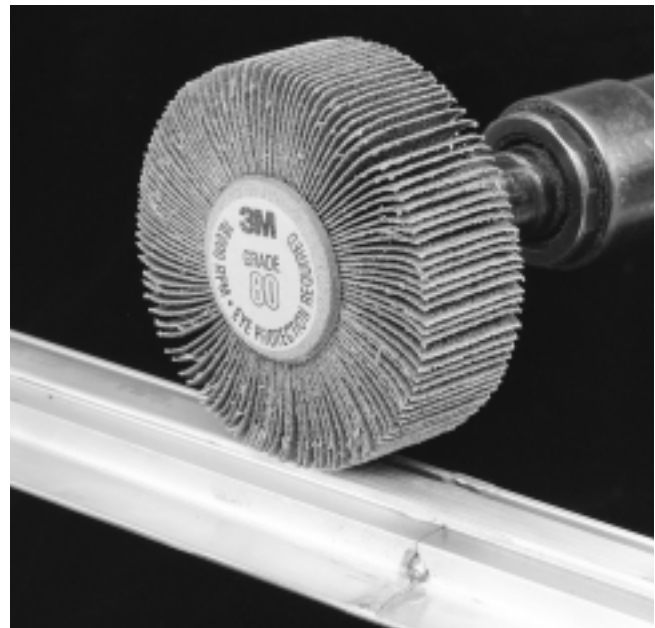
Weld removal and blending (above) – The 3M PG wheel removes, blends and finishes uneven welded surfaces of this aluminum aircraft component.
