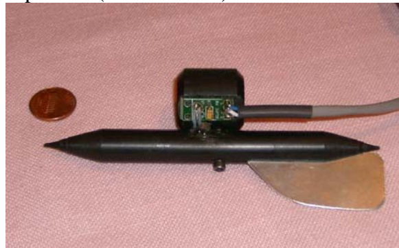
Board with cable and Hall sensor mounted off the side of PC board Note surface mount capacitor ( Yellow cube)
