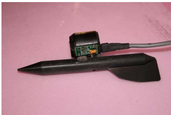
AOA Vane and Mount with Hall Sensor
