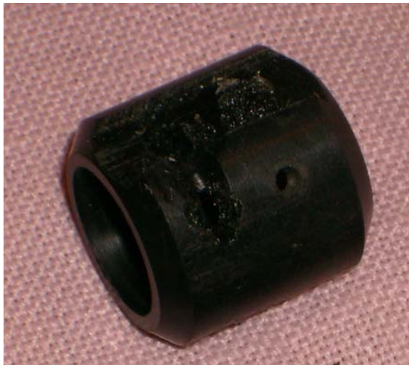
AOA Pitot Mount (Small hole holds Hall sensor)
