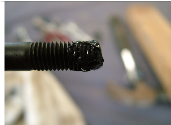
A little molly grease was added to the tip.
