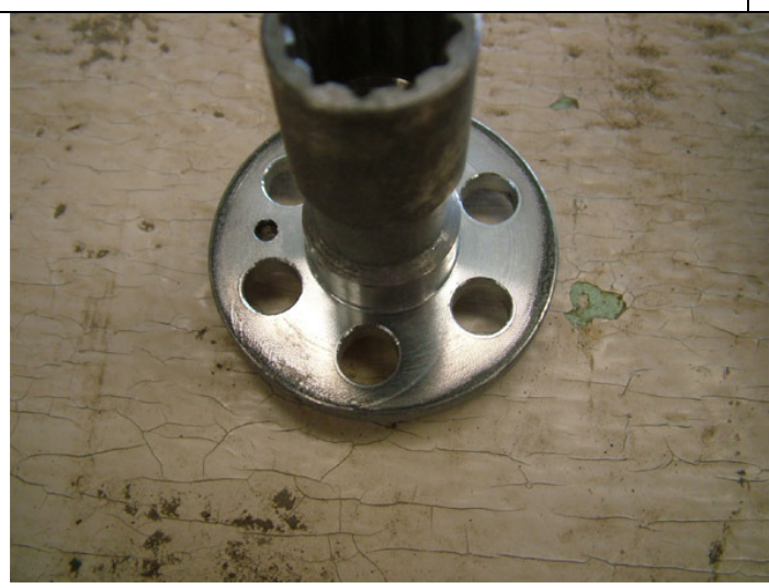
The vacuum drive which faces the flywheel.
