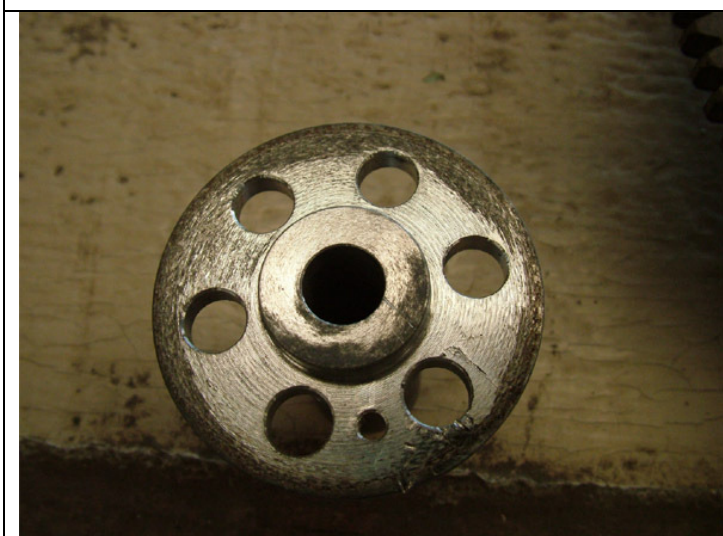
The back side of the vacuum drive.
