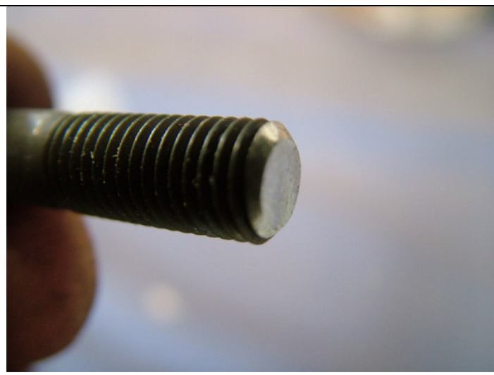
New bolts were cut and the tip finished.
