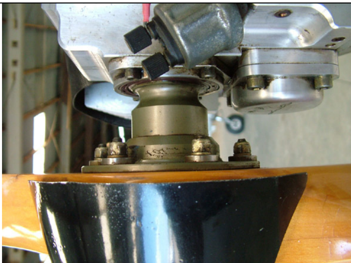
The prop extension, same on all three aircraft.
